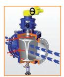
This IsoPlug image (left) shows the media (blue) with the plug in open position.
