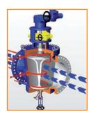
In this image, the second actuator has now been engaged and we can see that the plug is turning. Flushing (shown again as red lines) will now take place in, around, above and below the plug.
