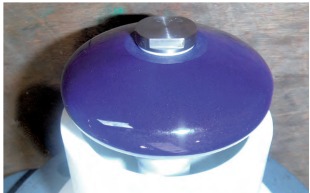
Glass Disc with Temperature Sensor underneath a tantalum cap
